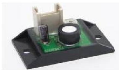
FIG 5. SENSOR MODULE FOR COMBUSTIBLE GASES
