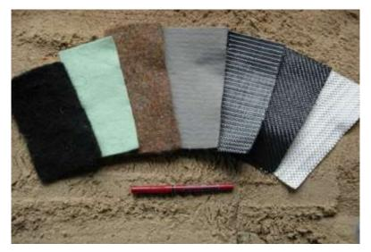
There are two principal geotextile types, or structures: woven and nonwovens. Other manufacturing techniques, for example knitting and stitch bonding are occasionally used in the manufacture of specialty products.
