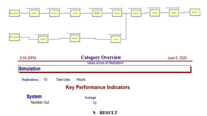
Implementation of future state resulted in reduction of total lead from 132.3 hours to 50.30 hours, giving a 61% reduction in lead time.
