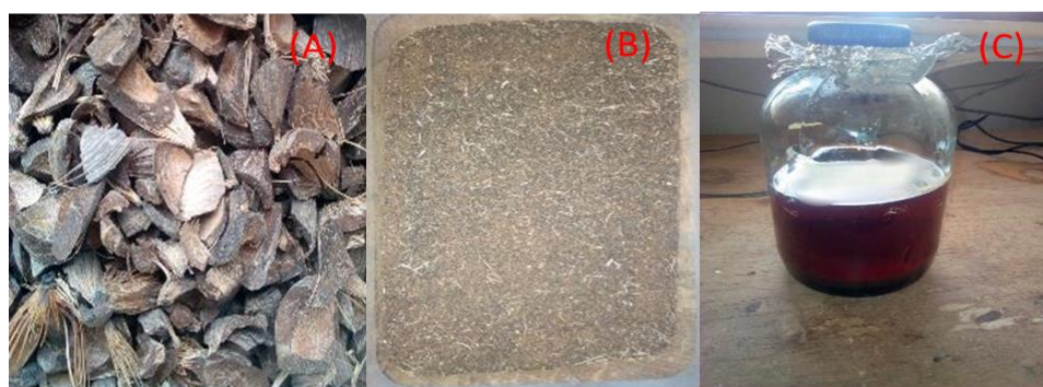
Figure 1: (A) Freshly collected Elaeis guineensis shell waste sample, (B) Pulverized sample, (C) Macerated sample
