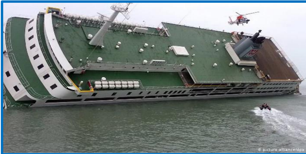
Fig. (7): A photo of M/V SEWOL before sinking, the photo shows that all life rafts were unused. Source: The New Yorker (2019)
