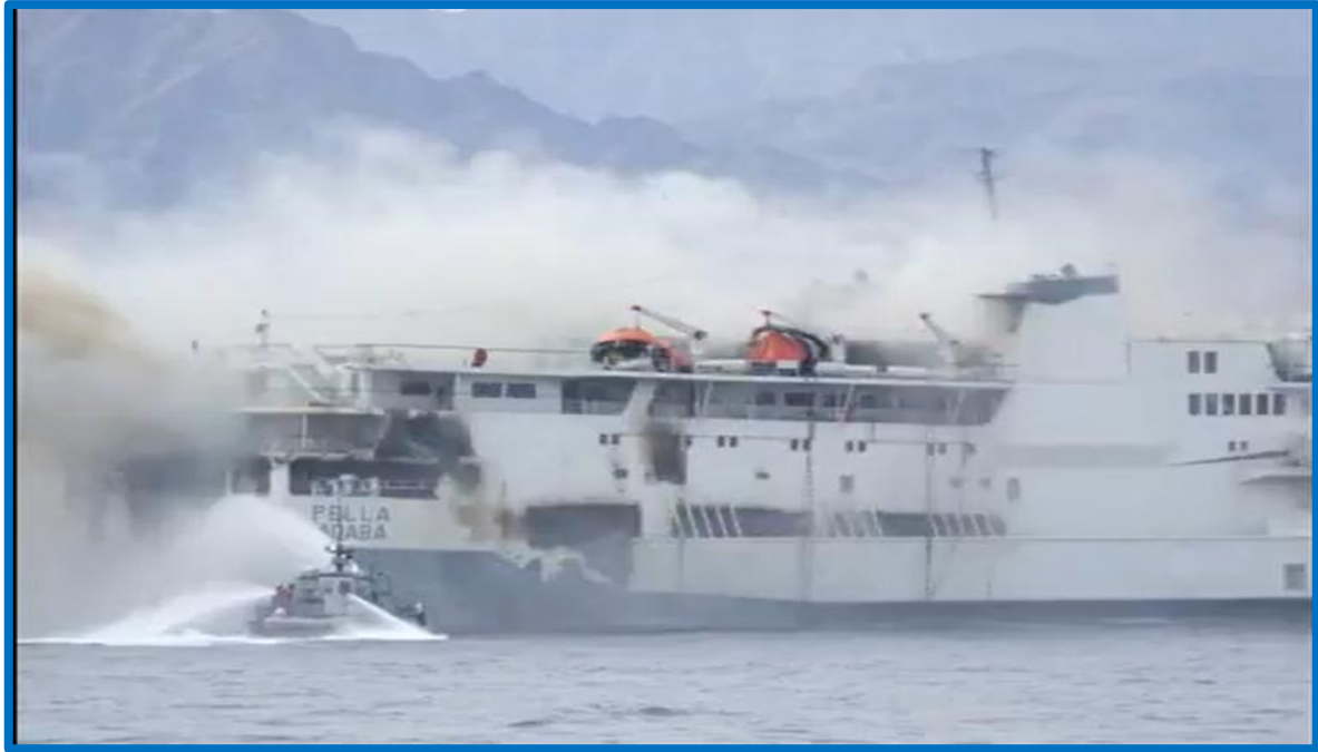
Fig. (6): Photo of unused life rafts due to the spread of the fire on starboard side. (Jordan maritime authority administration, 2008).
